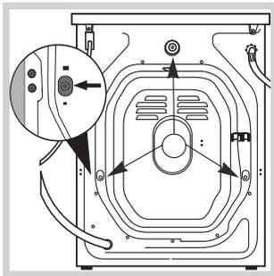
3. Remove the **3** protective screws (used during transportation) and the rubber washer with the corresponding spacer, located on the rear part of the appliance (see figure).
