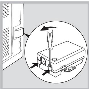
1 Open the terminal board by inserting a screwdriver into the bottom tabs of the cover. Use the screwdriver as a lever by pushing it down to open the cover (see diagram).
