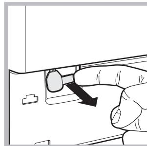
4. Using the tab shown in the figure, pull outwards until the plastic brace comes away; pull it downwards until you hear a "click", which indicates that the door is unlocked;
