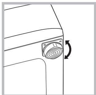
2. If the floor is uneven, the feet of the appliance may be adjusted until it reaches a perfectly horizontal position (the angle of inclination must not exceed 2 degrees).
