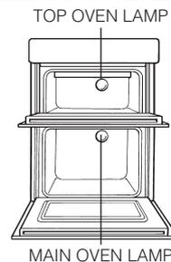
**Warning: To avoid electric shocks - please ensure that the electricity supply to the appliance is switched off and the appliance is fully cold, before cleaning lamp lens.**
